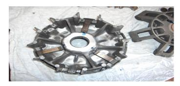
The 3 stock and 3 adjustable weights are alternating. The 3 stock are 120 degrees apart, as are the 3 new ones. – Every second one is replaced. THIS IS THE ONLY CONFIGURATION THAT 3 WEIGHTS CAN BE REPLACED.
