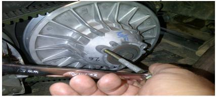
Using the Clutch spreader bolt from BRP (A fully threaded M8 X 1.25 bolt can be used ) spread the secondary make slack to remove/install the belt.
